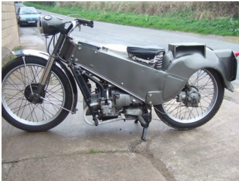
Folded/pressed steel sheet frame: Velocette LE
