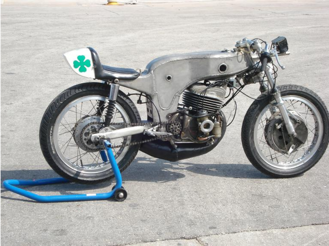
Fabricated aluminum sheet beam/monocoque frame: Ossa 250GP 1968
