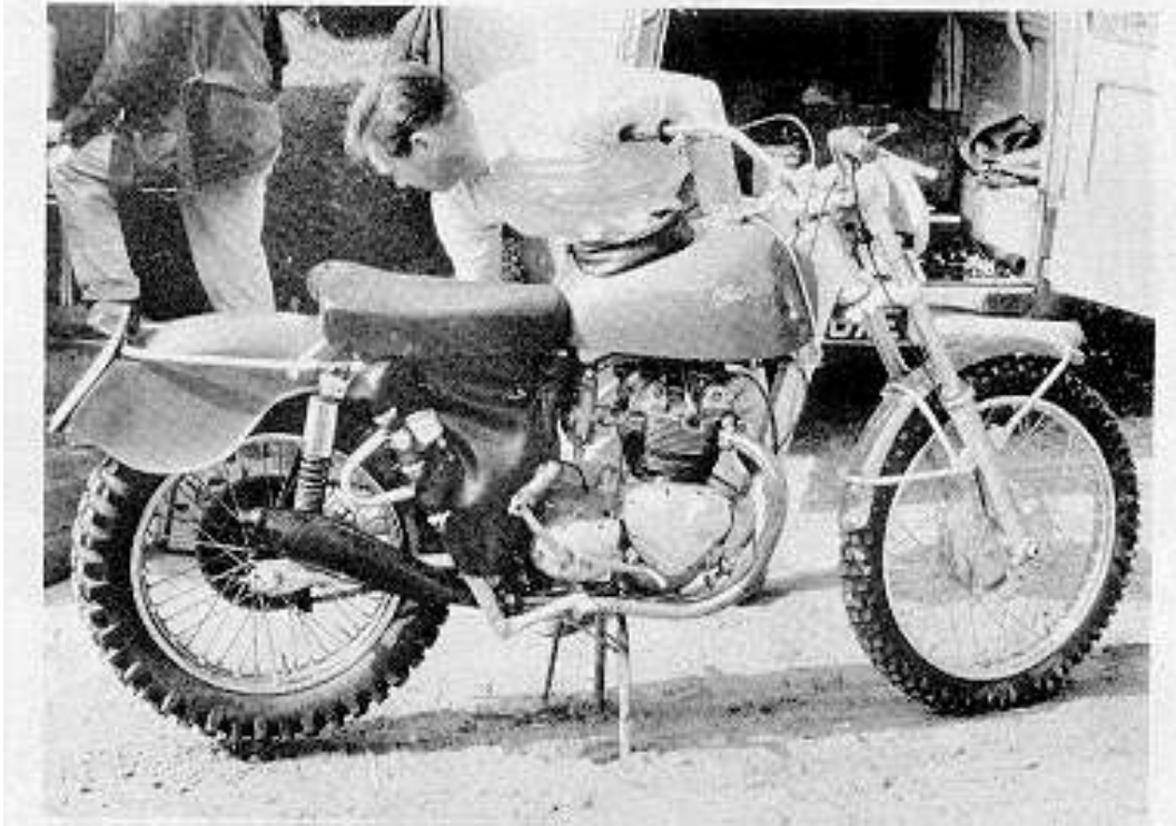
Square steel tubing: Butler Triumph circa 1966, source either Motorcycle Sport or one of the UK weekly papers.
