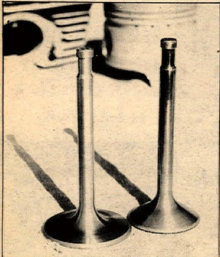
Right is a stock valve. Compare it with the replacement valve on the left. It began as a Chevrolet part.
