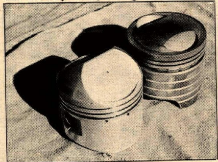
Right is the stock Eagle piston. Left is the replacement part constructed from an M.C. forged BSA Victor piston. The crown has been welded up and machined to its present size. Notice the heavy knurling on both skirts. Kyle lets his pistons fit loosely, relying on rings for compression.
