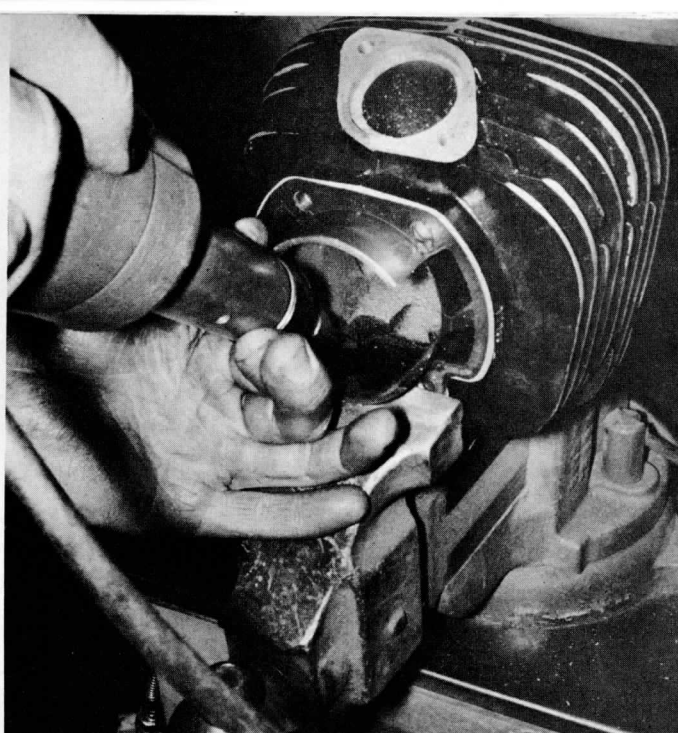
Modifying 2-cycle cylinder ports not only takes special tools but a special talent, also.
