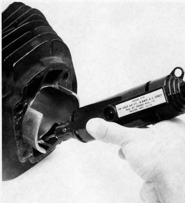
6. A high-speed grinder (20,000 to 30,000 rpm) with a milling bit is best for the initial trimming-to-shape inside the ports.
