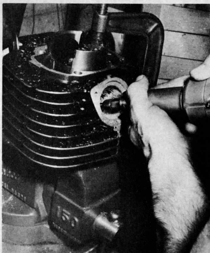
C-clamp to vise is a novel way to obtain good working positions. The exhaust hole is getting some extensive grinding.
