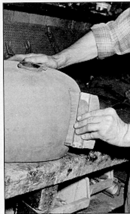
5: ... and checks the profile with a gauge against a Thruxton tank.
