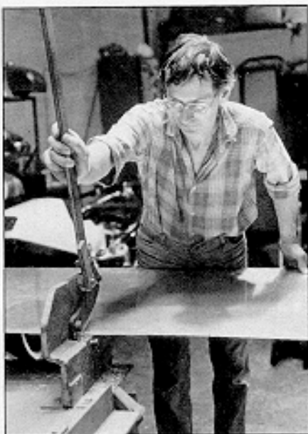
2: Even the large guillotine will cut around the outside curves.
