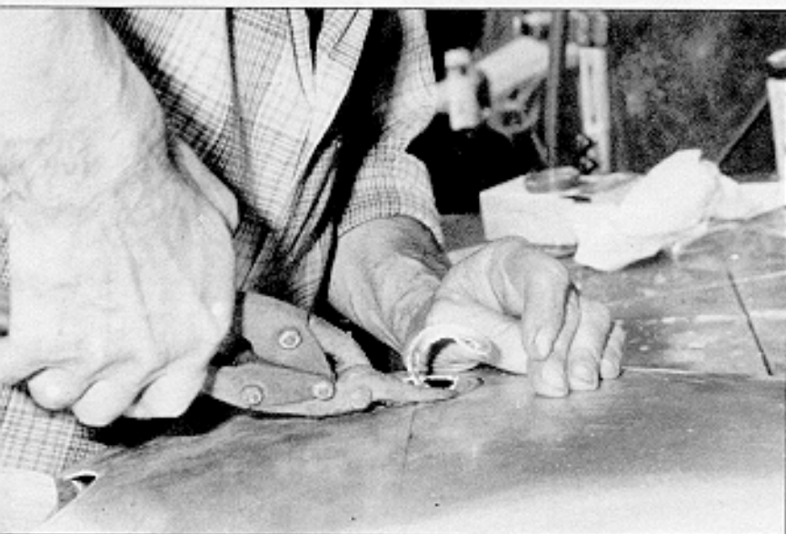
He cuts the hole with tinsnips and the job's finished apart from the petrol tap and front mounting lugs. Tomorrow's job!
