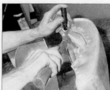
26: He has to use a screwdriver to pull the 'tunnel' into place.
