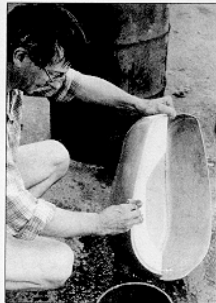
9: The tank must then be washed.
