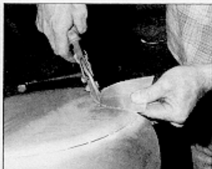
10: The tank is cut away where it will fit around the steering head.
