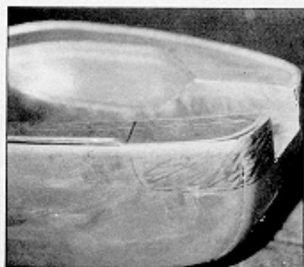
27: The area that must be cut away to clear the GP carburettor.
