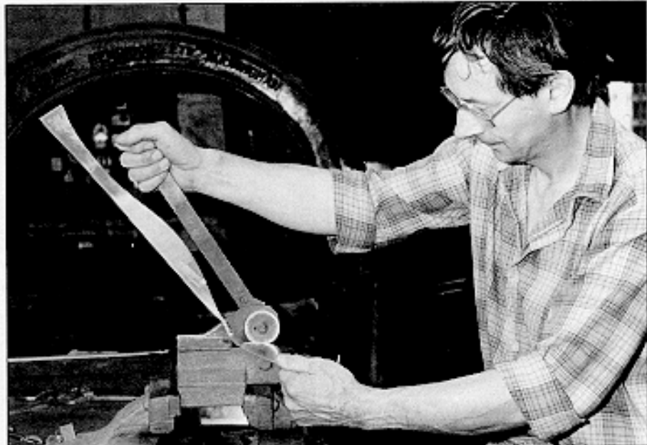
3: Inside curves are cut out with a smaller guillotine.
