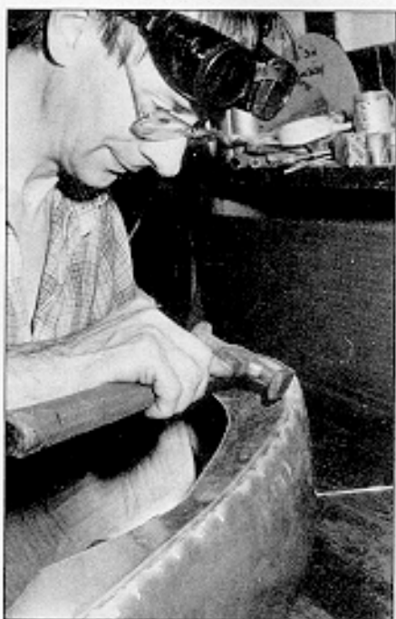
17: The heat distorts the side. Pete corrects it with a hammer.
