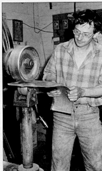
4: Pete shapes the tank top with the 'wheel'...
