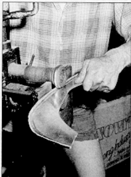
15: Throwing up a ridge on the bottom of the tank.
