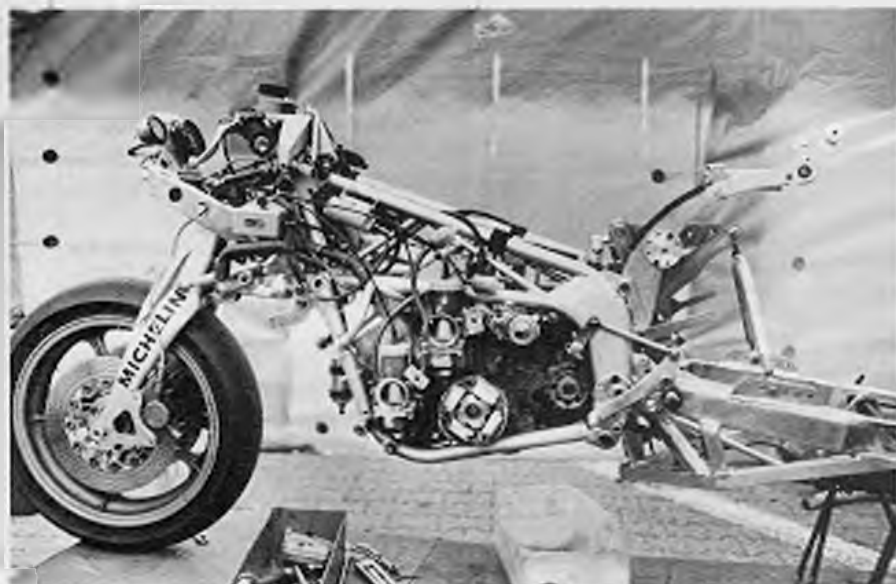
The Elf design uses an asymmetrical steering upright. The wheel is dish'd so that both ball joints lie in the wheel's central plane. A line drawn through the two joints defines the steer axis, which, owing to the dish'd wheel, can be offset to the rear of the axle as in tele designs.
