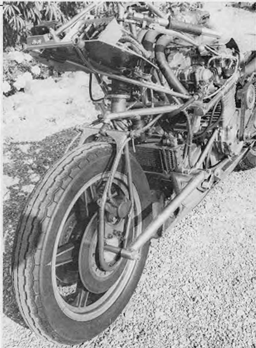
The Simms up-and-down fork places the large-diameter riders at the top, where the greatest stiffness is required.
