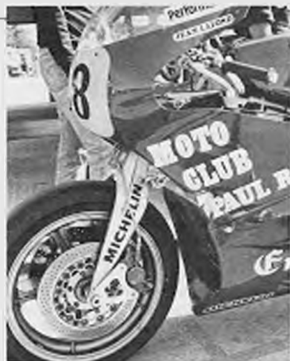
The Elf design uses an asymmetrical steering upright. The wheel is dish'd so that both ball joints lie in the wheel's central plane. A line drawn through the two joints defines the steer axis, which, owing to the dish'd wheel, can be offset to the rear of the axle as in tele designs.
