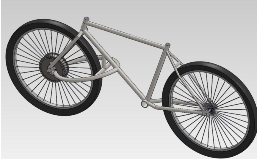
Figure 41: CAD Frame and complete wheel assembly
