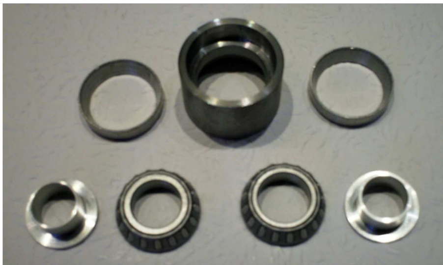
Double Wishbone bearing holders Small bike bearings -with Steel reducers to 12mm
