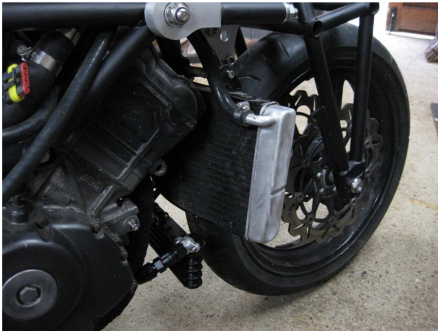
Earl's oil hose and connectors. Earl's do steel bosses which I had welded to the stock engine take-offs
