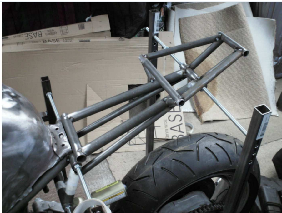
Cut tubes and made a jig for the Hossack forks
