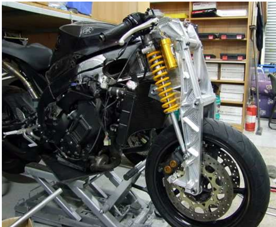
Final R1 girder design in 6061 aluminum
