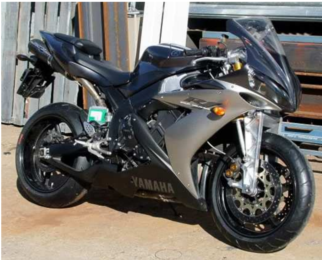
Yamaha R1 with aluminum girder front suspension from SuspensionSmith of Australia
