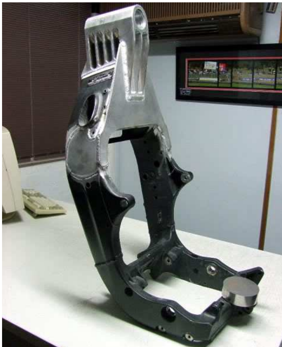
Longer steering head welded on R1 Frame
