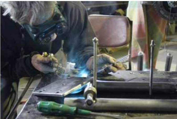
Brazing on the axle bobbins
