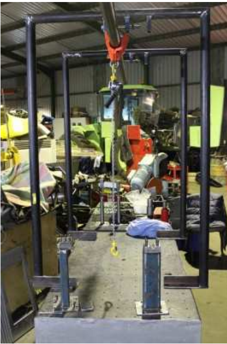
The setout table and jig frame that will be used for all development, fabrication and testing forces
