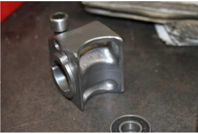
Front axle mounts ready to be welded on to the leading link
