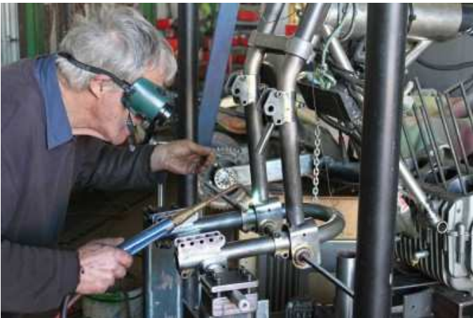
John tacking the pivot saddles to the chrome moly down tubes
