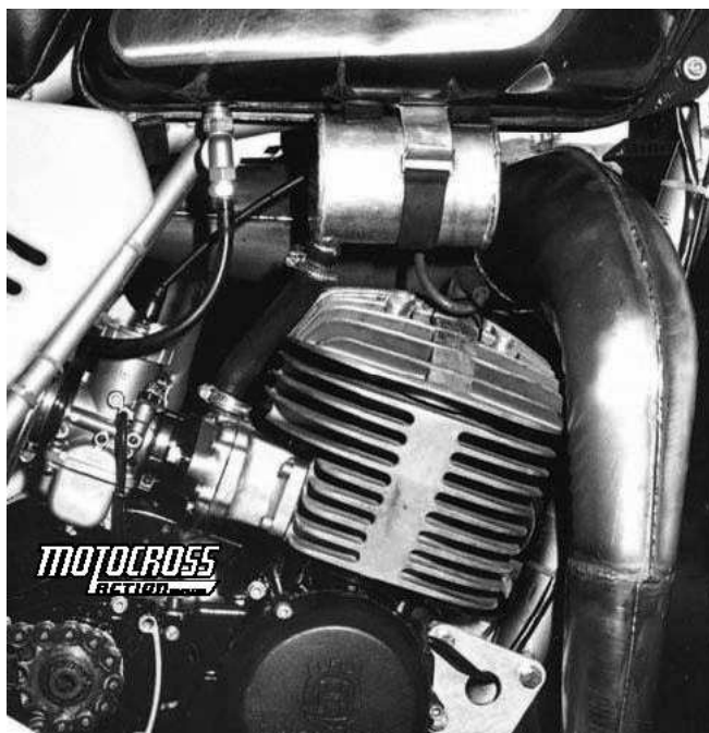
As an aftermarket part, this Pro Circuit Husqvarna has an aluminum boost bottle attached to a rubber hose. The hose fits between the carb and reed block.
