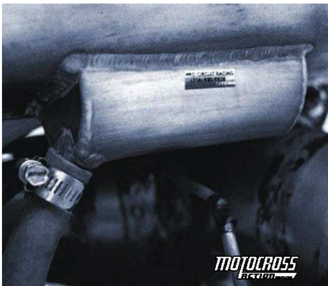
Andy Jefferson's Pro Circuit Husqvarna had the boost bottle built into the aluminum Husqvarna gas tank.
