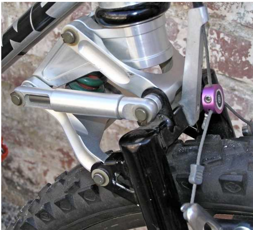
Horst Leitner took the linkage elements of his motocross fork and miniaturized it to produce the AMP Research B4 mountain bike fork. It is a four-bar linkage that folds on impact. The tiny aluminum shock is a thru-shock (in that the shock shaft come out of the opposite end of the shock body) and a pull shock (the shock is extended under movement instead of compressed). The spring is inserted between the linkage (and is visible at the back of the fork).
