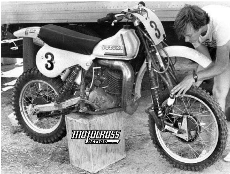
The Ribi Quadrilateral fork wasn't about suspension travel as much as geometry change.
