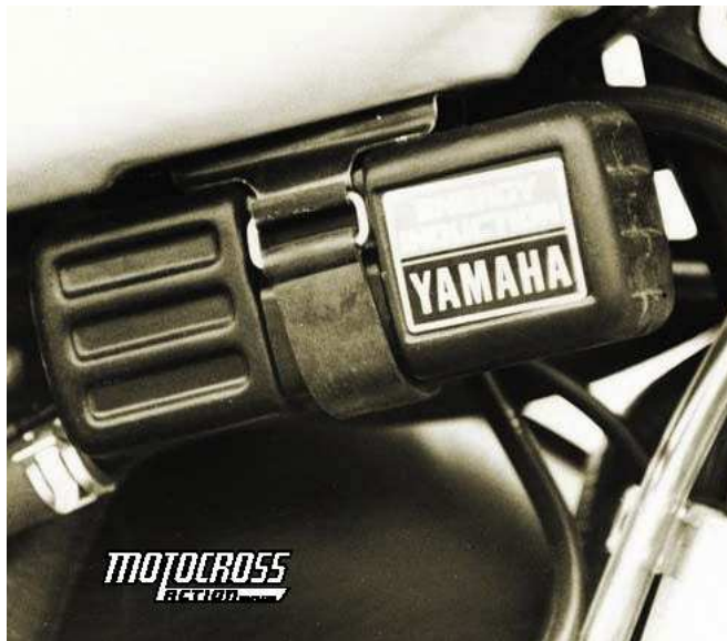
Yamaha put boost bottles on their bikes as an OEM part.
