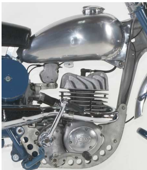
The British-built Greeves motocross bike had a cast, one-piece, aluminum head tube and down tube and stamped engine cradle starting in 1954.
