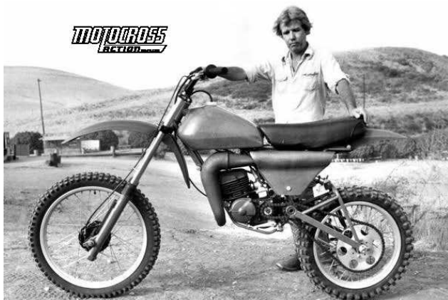
Dave Thompson didn't just install a jackshaft system, he turned his 1979 CR125 into an Fox AirShox-equipped monoshock.
