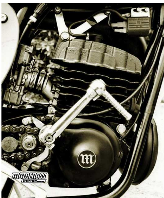
The wrinkles increase the surface area of the cylinder's fins.
