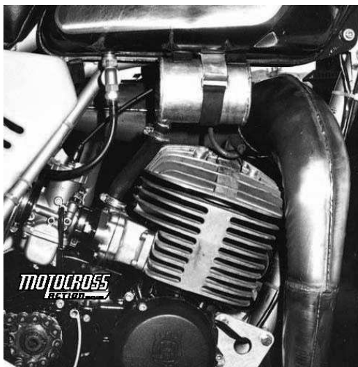
As an aftermarket part, this Pro Circuit Husqvarna has an aluminum boost bottle attached to a rubber hose. The hose fits between the carb and reed block.
