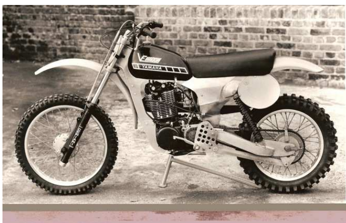
Back in the 1977 British speedway and sidecar builder Hagon built monocoque aluminum motocross frames to accept a wide variety of four-stroke engines.
