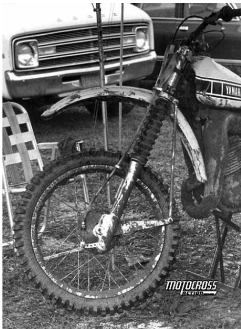
Although the mechanical No-Dive system may look Rube Goldberg, it was used on the works bikes of Roger DeCoster, Broc Glover (shown here) and Kent Howerton.
