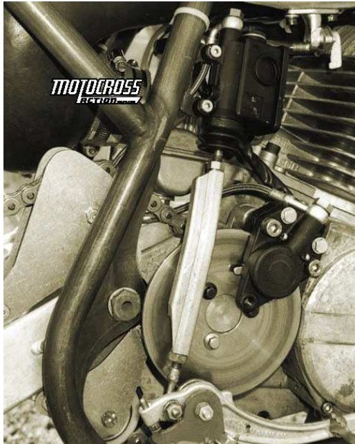
ATK's rear brake was mounted on the countershaft sprocket.
