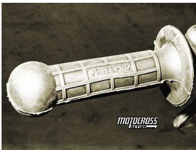
The Jones Ball Grip was designed to keep you hand from slipping off the grip and to provide a massage ball to lessen arm pump during long races.
