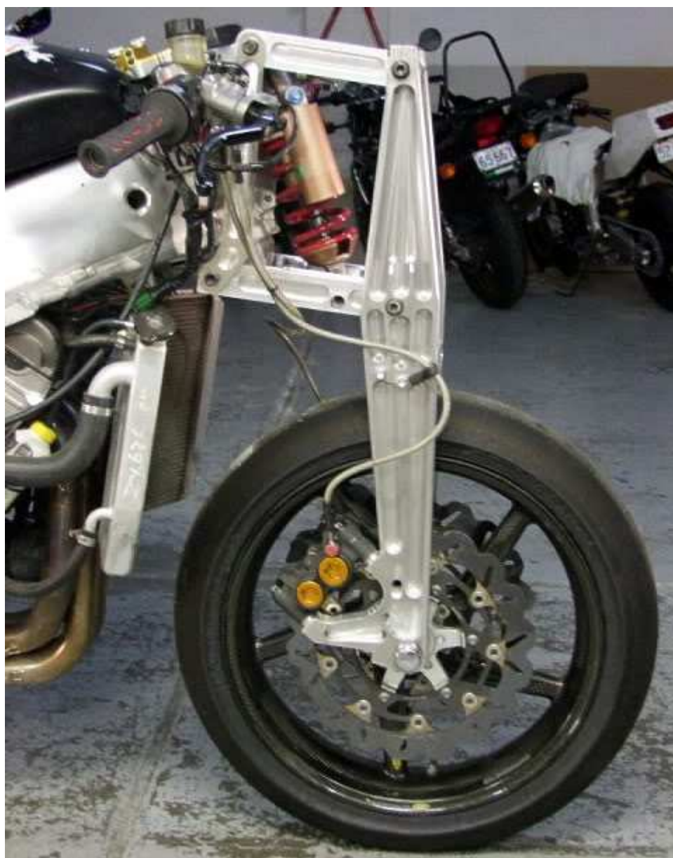
First girder prototype on FZR400 with Honda CBR 919 engine
