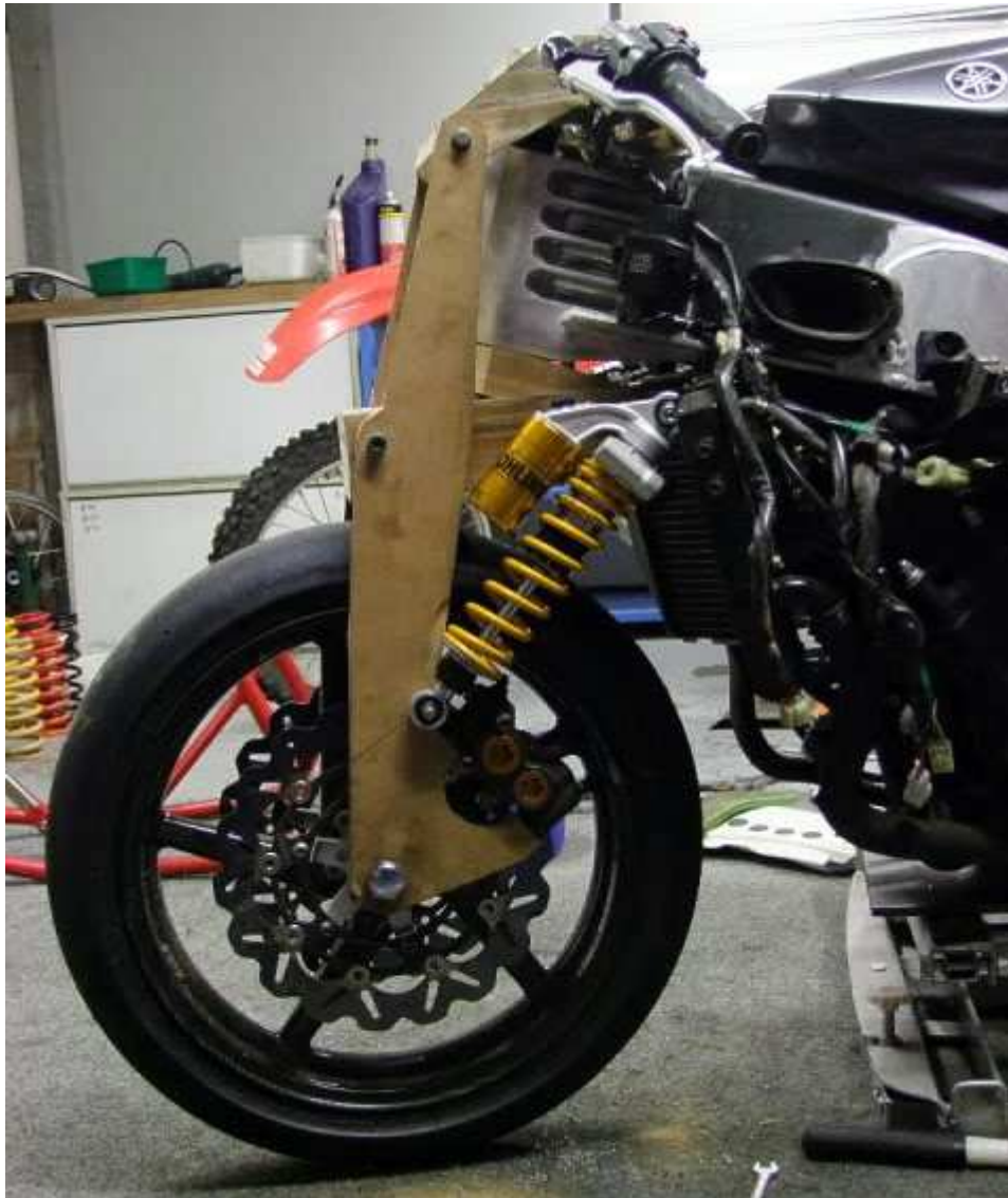
First R1 girder prototype in wood
