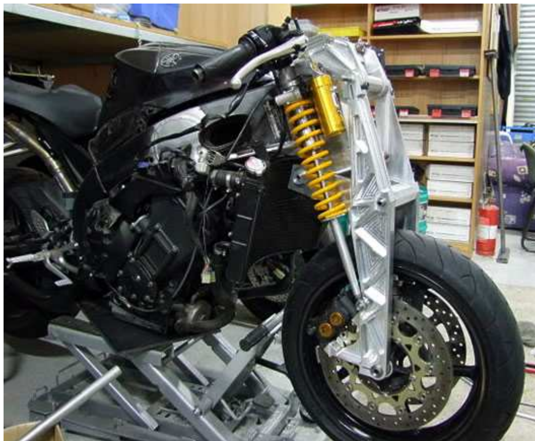
Final R1 girder design in 6061 aluminum
