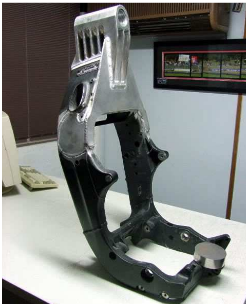
Longer steering head welded on R1 Frame
