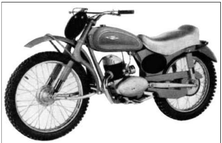
The Moto-Cross Mark 5 which was powered by a Villiers 200c.c. 7E engine.
