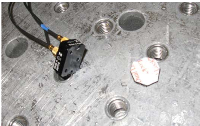
Test accelerometer and \frac{3}{4} " diameter 3M Dual Lock patch before mount
