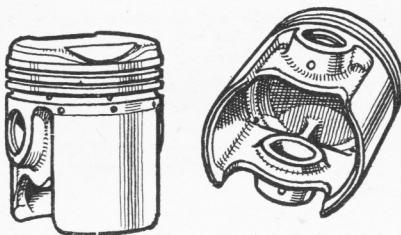
Forged-type pistons of slipper design were adopted for the original Tiger 100, which is the super-sports edition of the "Speed Twin." It had a rather higher compression ratio
