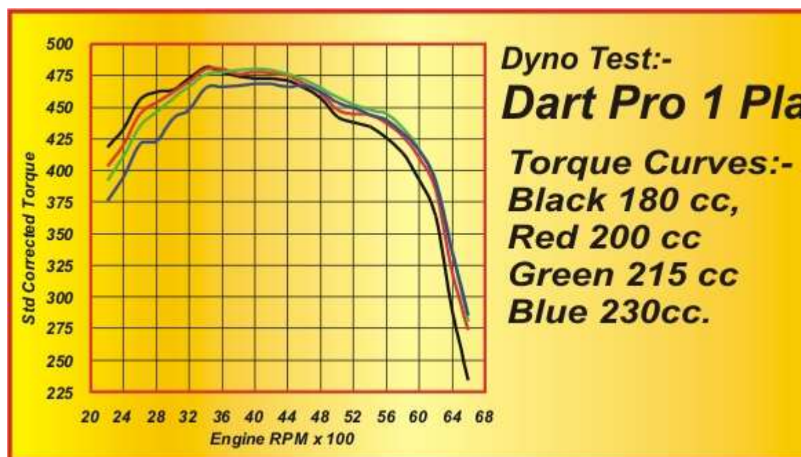
Fig 3. The results here clearly show that smaller, higher velocity ports, favor low speed results also show that going too big (blue curve of 230 cc port) on the ports, for the produces worse results almost everywhere in the rpm range.
