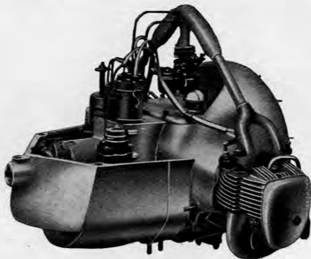
FIG. 5. Air-cooled four-cylinder engine of the Tatra 30 type.
