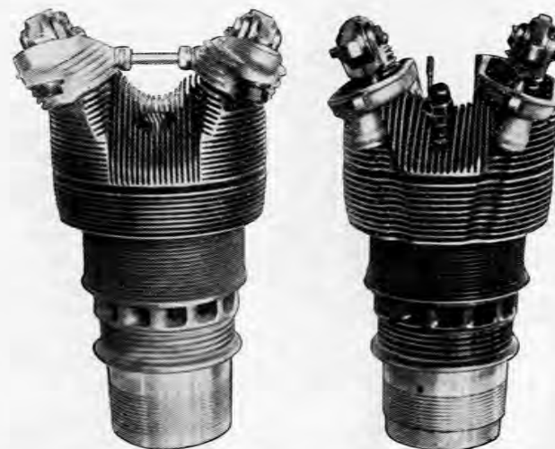
FIG. 352. Old and new design of the cylinder of the ZOD engine.
