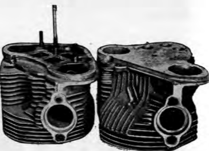
FIG. 219. Two differently finned cylinder heads of the Tatra 603 engine viewed from the spark plug side.
