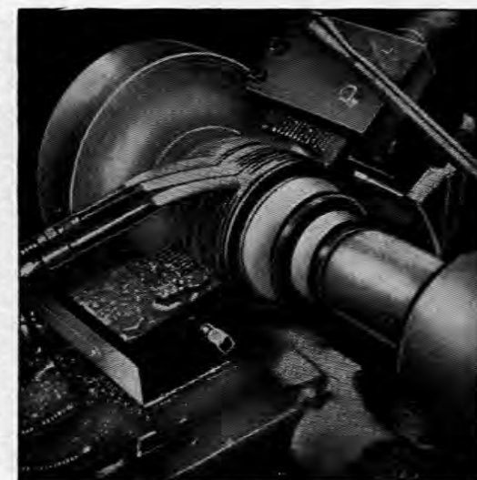
FIG. 244. Machining of fins of an air-cooled engine cylinder.
