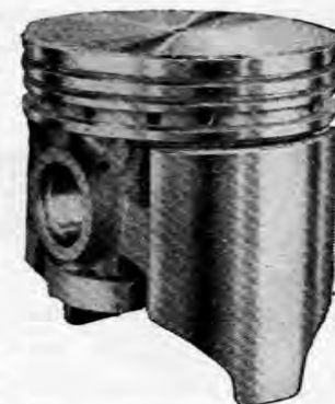
FIG. 322. A modern piston of a high-speed engine.
