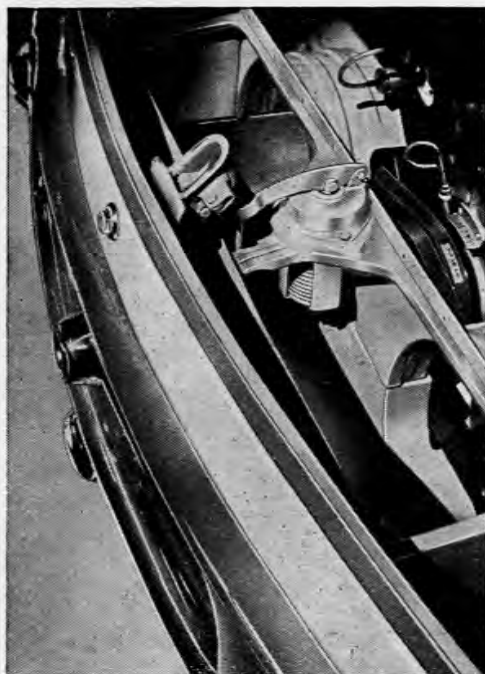
FIG. 123. View of the thermostat operating the cooling control flap.
