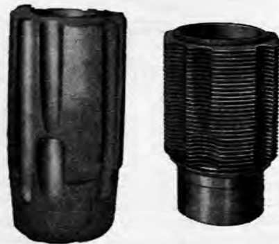
FIG. 245. Cylinder of the Tatra 111 compression-ignition engine prior to and after machining.
