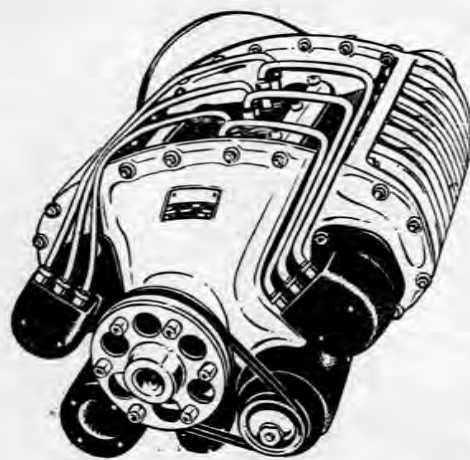
FIG. 355. Two-stroke three-cylinder engine with opposing motion pistons and reduction gear.
