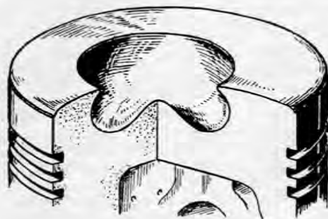
FIG. 41. Well designed combustion chamber in piston of oil engine.
