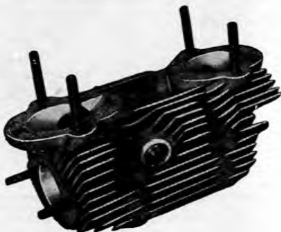
FIG. 221. Cylinder head of the Tatra 603 engine with inclined finning. Note the poorer finning in the region of the spark plug.
