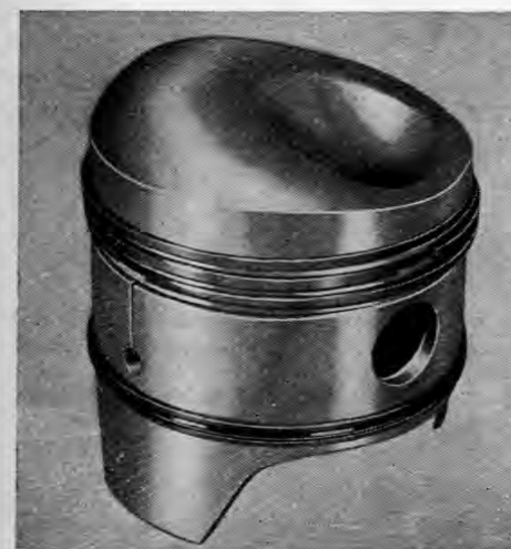
FIG. 184. Experimental piston with well shaped crown for a hemispherical combustion chamber.
