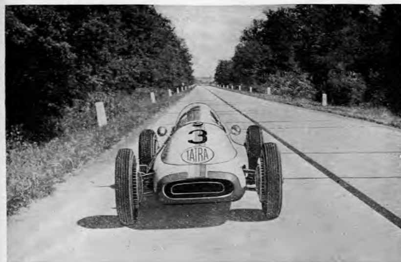
FIG. 19. Tatra racing car with air-cooled rear engine.
