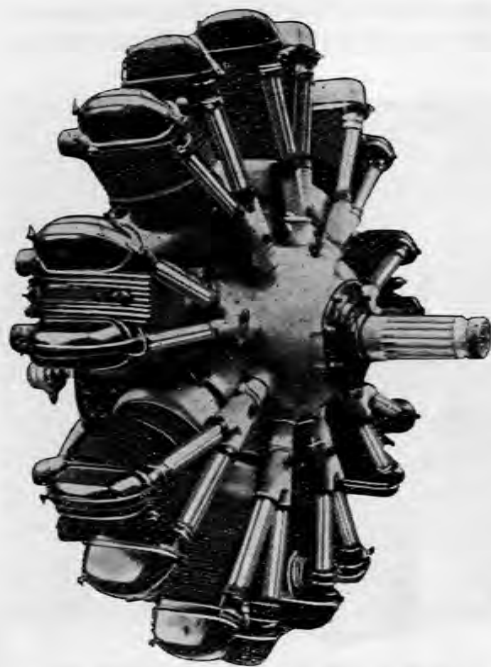
FIG. 22. Air-cooled two-stroke aircraft engine of the ZOD type.
