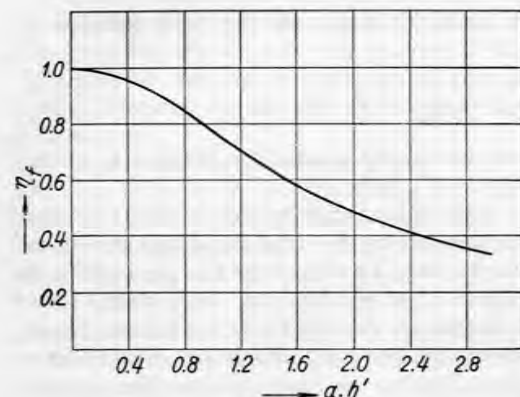
FIG. 54. Efficiency of cooling fins according to equation (21).
