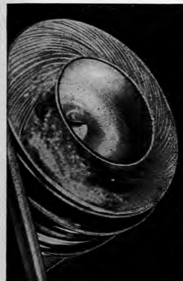
FIG. 226. Double compression turbulence in the toroidal injection chamber in the piston of the Tatra compression-ignition engine.
