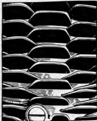
FIG. 252. Intermittent finning of the cylinder of the Triumph motor-cycle engine.
