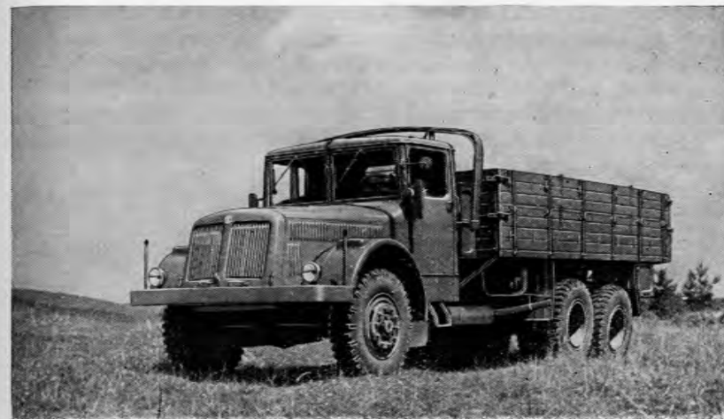
FIG. 9. The ten-ton Tatra 111 is fitted with a twelve-cylinder air-cooled engine.
