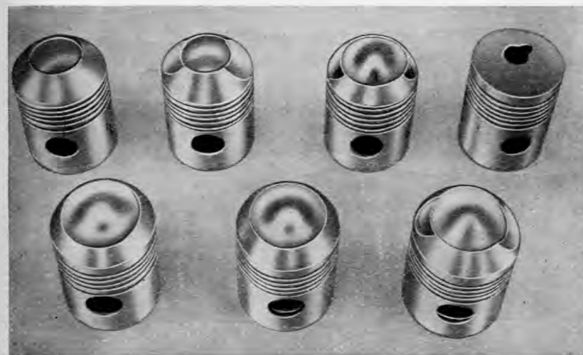
FIG. 12. Development of piston combustion chambers in the Tatra oil engine of 110 mm bore.
