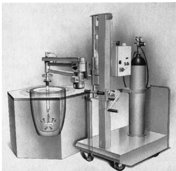
Figure 6.2 The Foseco Mobile Degassing Unit.
