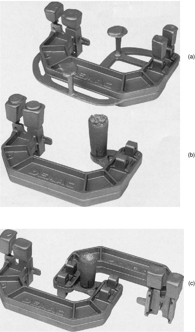
Figure 8.7 (a) Sand cast aluminium casting using standard running system. (b) Casting made using the KALPUR direct pouring sleeve/filter unit. (c) Optimised direct pouring system.
