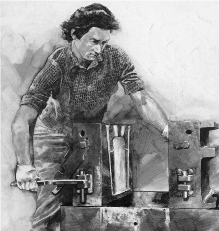
Figure 10.5 A manual gravity die set.
