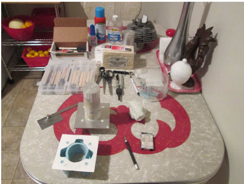
Silicone transfer port mold showing the lower cylinder-deck face where the transfer port windows will meet the crank case...
