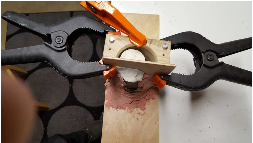
Wood, bondo, and clay are used to make a follower board and establish the parting line...
