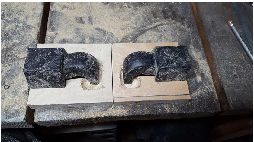
Setting up follower boards for the main transfer port core-patterns...
