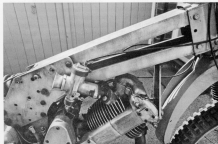
The Amal remote needle TTS carburettor shows the age of the design, today it would definitely breathe through a large airbox instead of gulping the raw dusty air!
